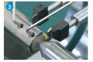
3. Set the back taper and adjust the insert height with screw the wedge screw
