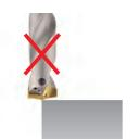
Irregular cutting resistance in plunging could cause fracture and deformation of the drill
