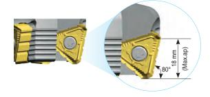
The serrations are effective with a depth of cut larger than 3 mm
