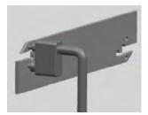
1) Insert the pin of wrench into the hole of blade.
