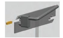
2 Clamp the insert on its seat after turning the handle to  $45^{\circ} \sim 160^{\circ}$  for loosening the seat.
