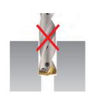
• Boring is not recommended due to wear and chipping in the corner of the insert
