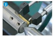
2. Rotate the reamer for the insert to touch the gauge
